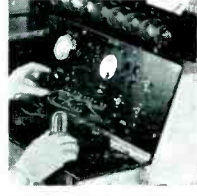
Finally, right before shipment tubes are again tested for shorts after a drop test.
