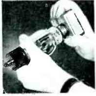
Torque test instruments check firmness of top cap assembly—
