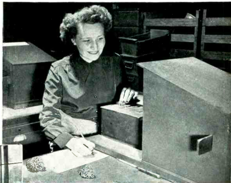
3 Every Carboloy Alnico Permanent Magnet is subjected to countless quality checks like this flux test to assure you of outstanding uniformity and performance.
