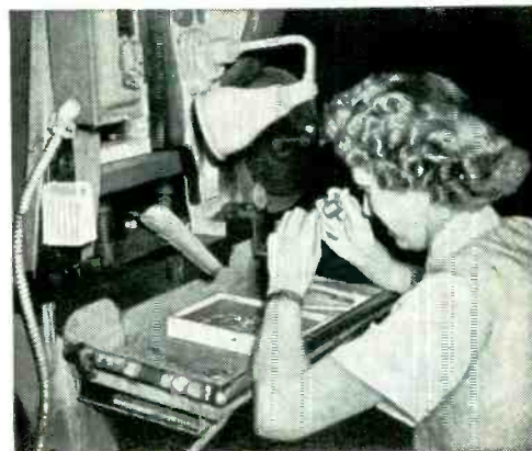
Part of inspection procedure on Lockseam Nickel Cathodes as they come off the production machine. Each cathode must undergo many rigid tests before being approved.
