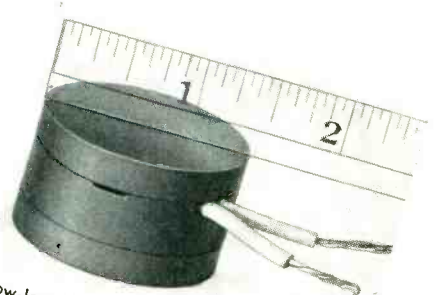
Low-loss inductor: inductance = 1 henry; Q = 400 at 30 kc. Extremely low-loss inductors and high-fidelity transformers are obtainable over a wide range of values and frequencies, using similar structures in various physical sizes.
