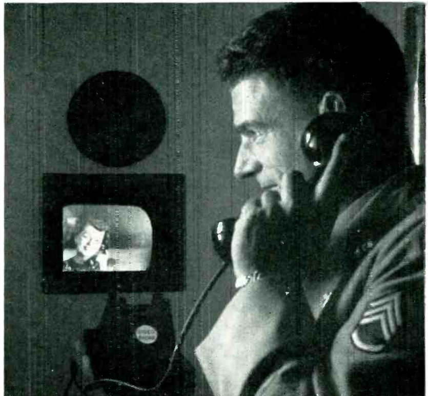
Video-Phone, a two-way television-telephone system
