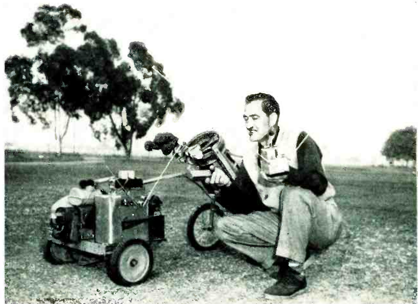
Jim Walker of Portland, Oregon, shown with a radio-controlled caddy cart and lawn mower which he designed. In his right hand is a small unit for controlling the machines from small distances. In his left hand is a unit for operating and controlling the machines for distances up to two miles
