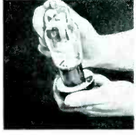
—critical inspectors check the alignment of filaments—
