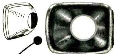
Rectangular TV envelope — mass produced of 1/8" 430 chrome iron, 24" wide, 16" high, 9" deep.
