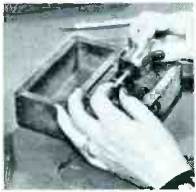
Cathode sleeves, like all other critical parts, are micrometer-checked—
