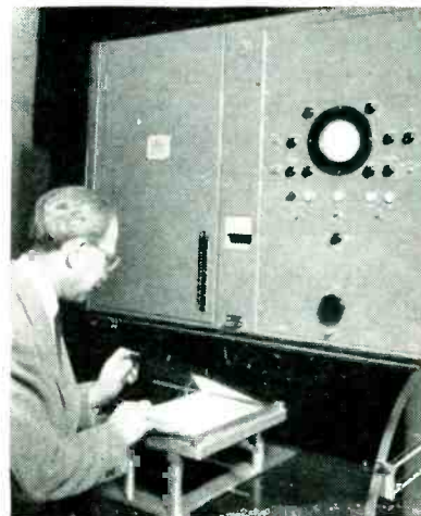
FIG. 1—Reader-transmitter of the test model of the new RCA facsimile system being prepared for operation by Roger Olden, research engineer. Operation of the transmitter is monitored by the oscilloscope on the right panel
